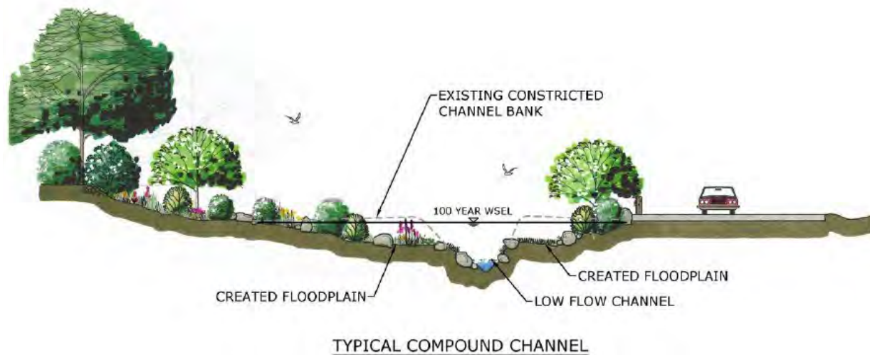
Figure 1-1: Cross Section of River Channel with Floodplains
