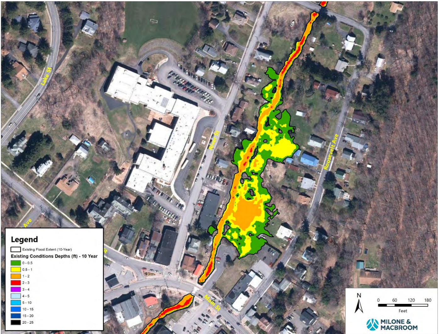
Figure 4-34: Existing 10-year depth grid mapping behind homes on Roosevelt Avenue
