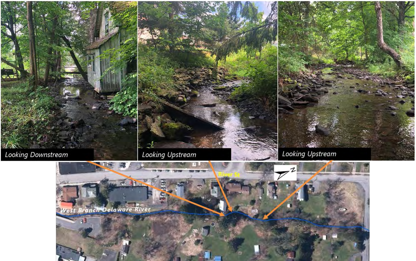
Figure 4-38: Photographs of the channel form illustrating the drastic change in channel top width as the stream approaches the area where regular flooding is being reported
