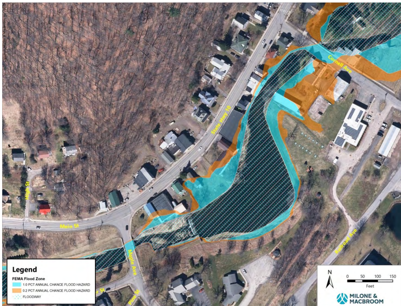
Figure 4-39: FEMA-mapped SFHAs of the WBDR behind properties along NYS-10
