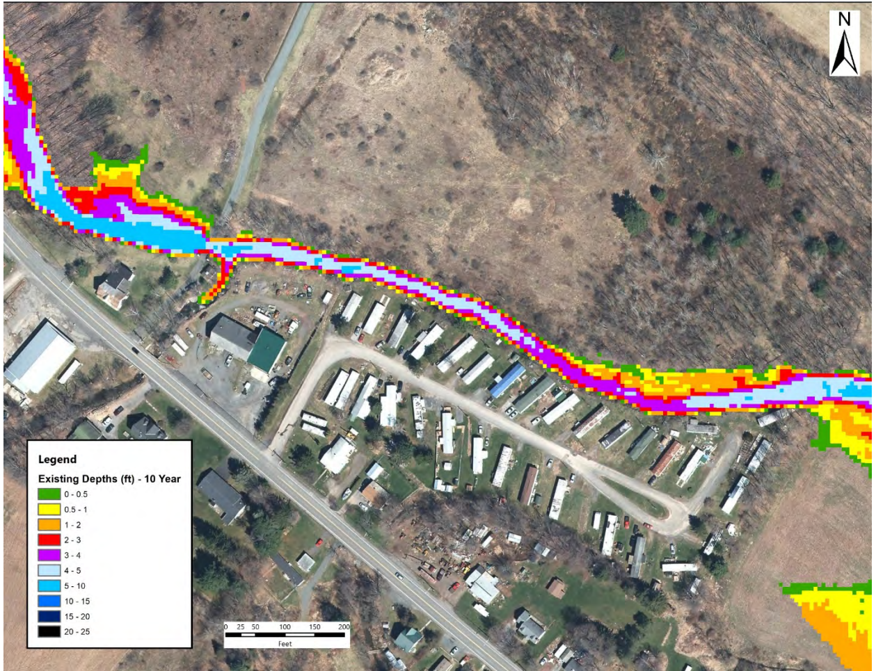
Figure 4-21 Depth Grid Mapping at Park Lane Homes – 10-Year Flood Existing Conditions
