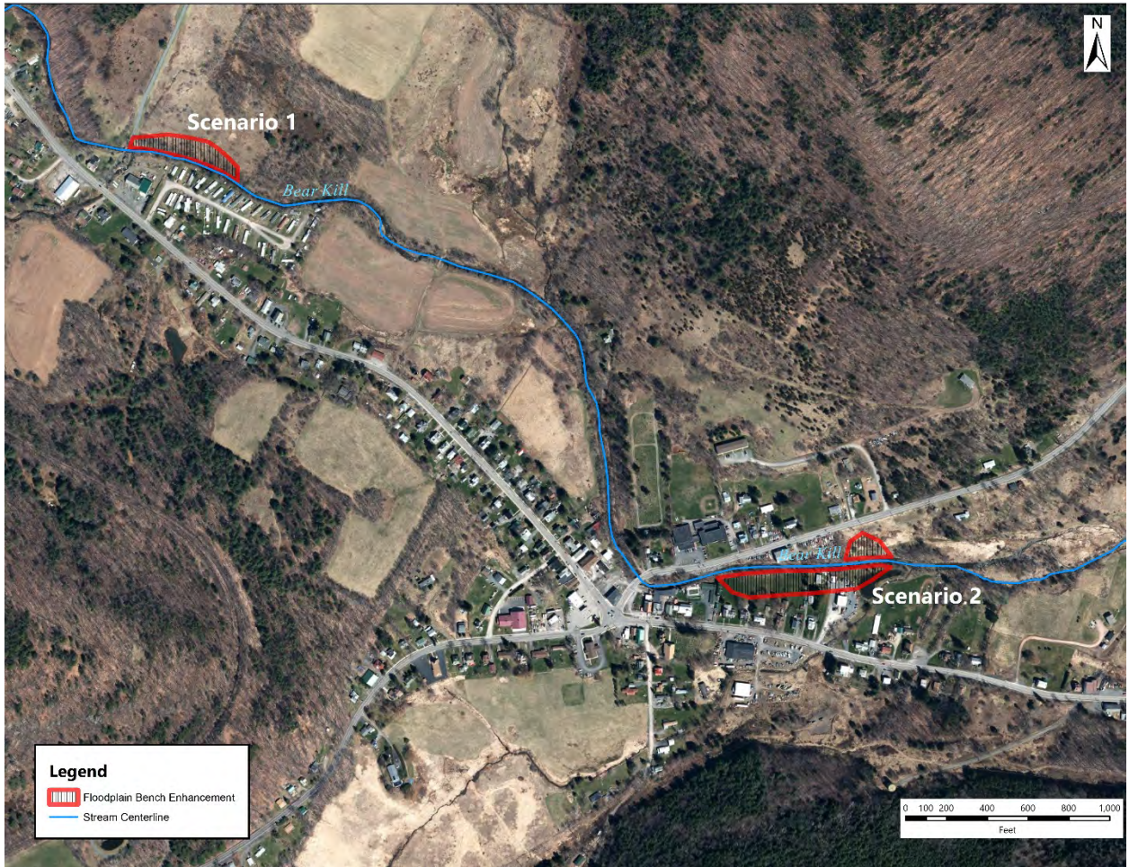
Figure 4-13 Areas of Floodplain Bench Enhancement along the Bear Kill, Hamlet of Grand Gorge
