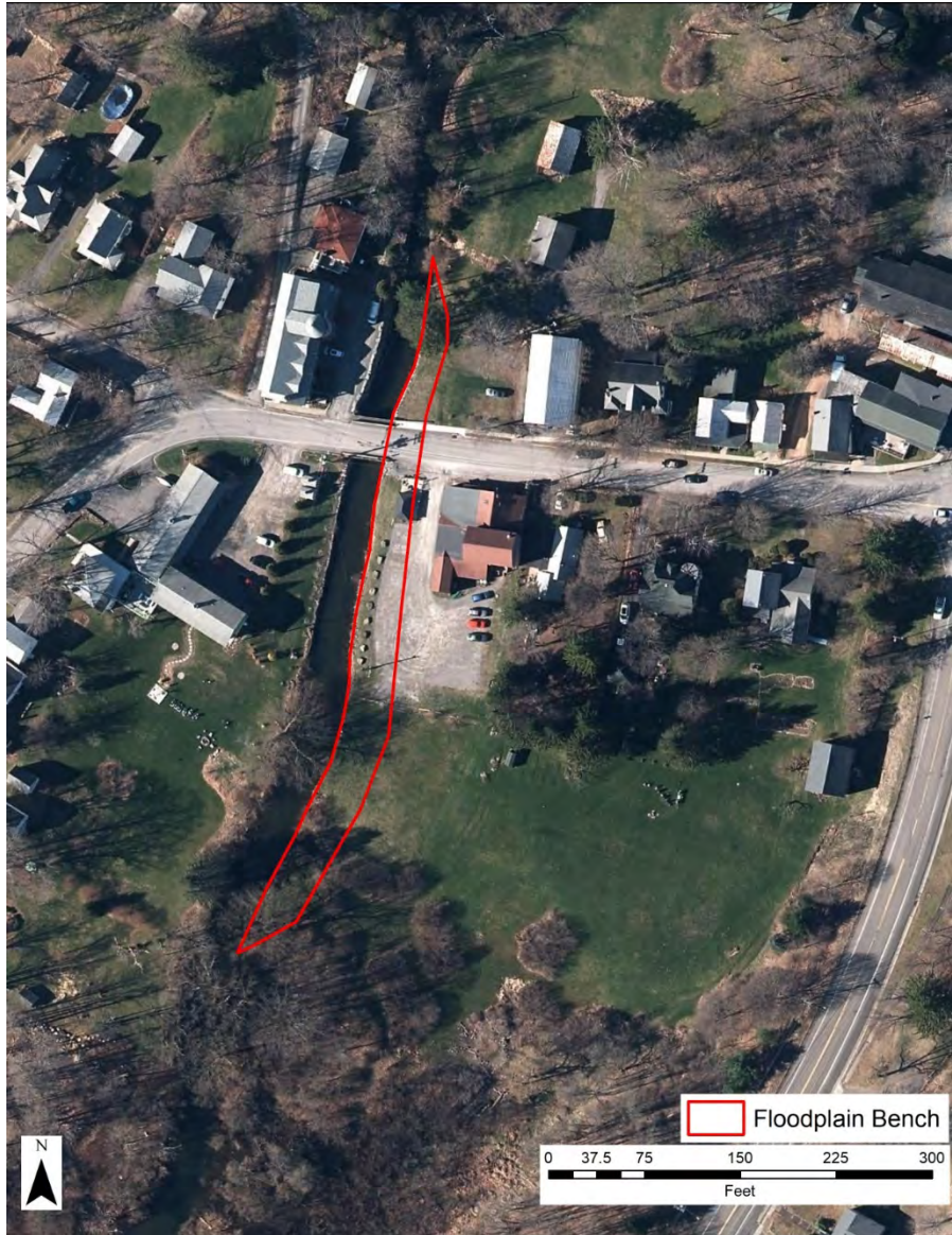
Figure 4-12 Floodplain Bench Enhancement along the EBDR at the Bridge Street Bridge, Hamlet of Roxbury
