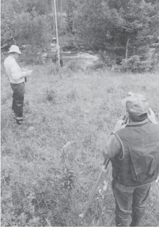
Figure 49. Good location for level setup.
