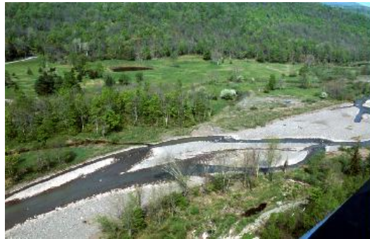
Photos of channel aggradation in the East Kill (left) West Kill (center), and upstream of an undersized bridge in the East Kill (right).
