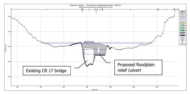
Figure 4-3: Representation of Alternative 4 in Hydraulic Model
