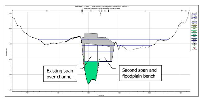
Figure 4-4: Representation of Alternative 5 in Hydraulic Model
