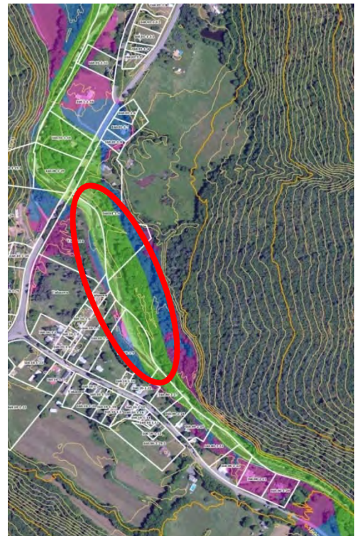
Figure 4-6: Area of Channel Migration and Bank Erosion
