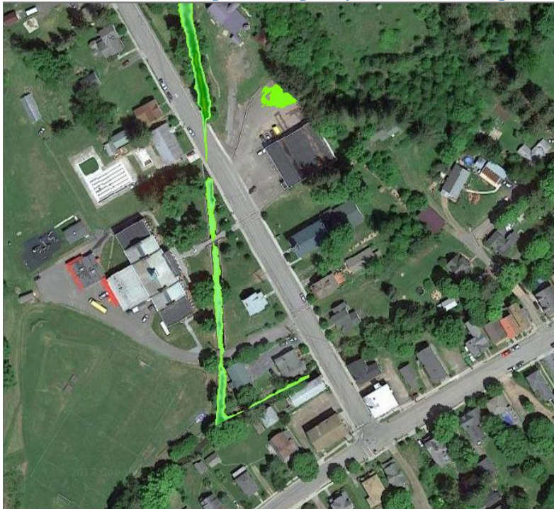
Figure 17. Inundation Area for the school retaining wall during a 50 year event for the proposed widened conditions.
