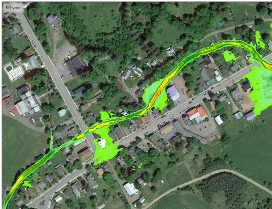
Figure 14. Inundation Area during a 50 year event for 33 Main St. to 103 Main St. – Proposed Conditions (Continuous Floodplain)
