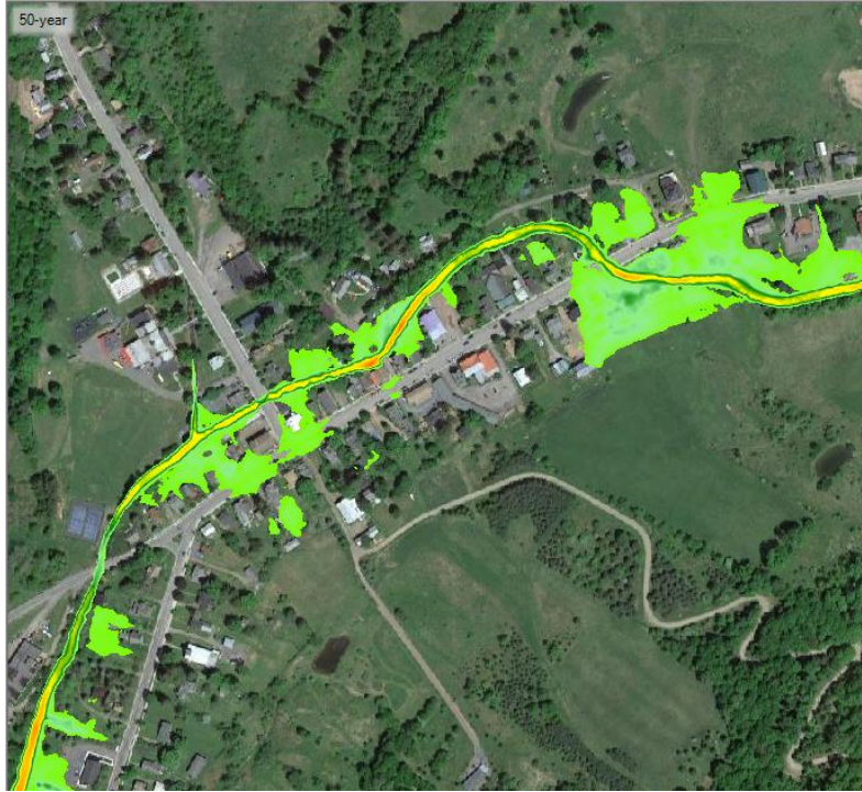
Figure 20. Inundation Area during a 50 year event through the hamlet for existing conditions.
