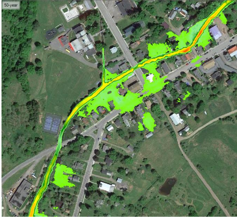
Figure 18. Inundation Area for the school retaining wall during a 50 year event for existing conditions.
