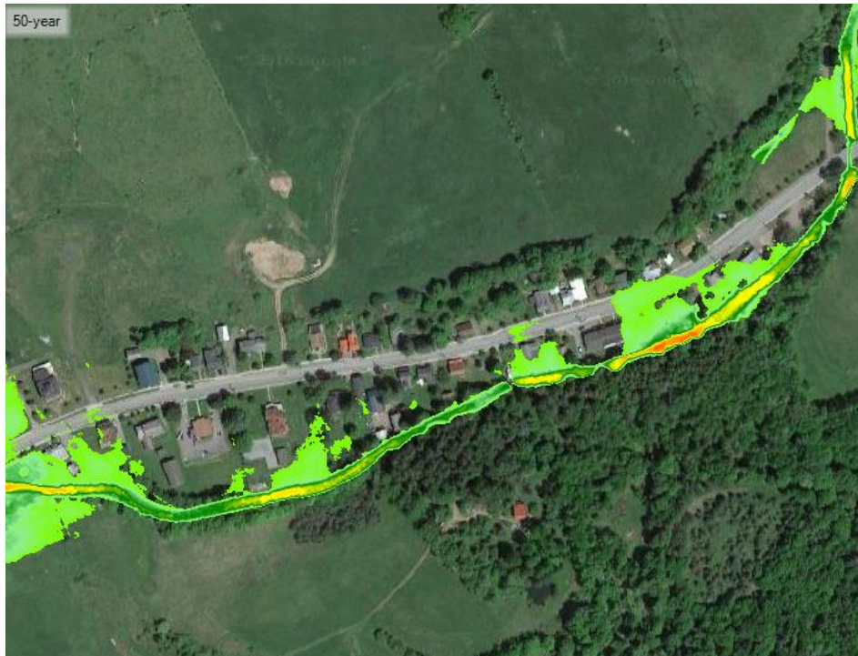
Figure 12. Inundation Area during a 50 year event for 288 Main St. to 506 Main St. – Proposed Conditions (Continuous Floodplain)
