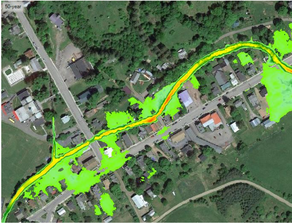
Figure 13. Inundation Area during a 50 year event for 33 Main St. to 103 Main St. – Existing Conditions
