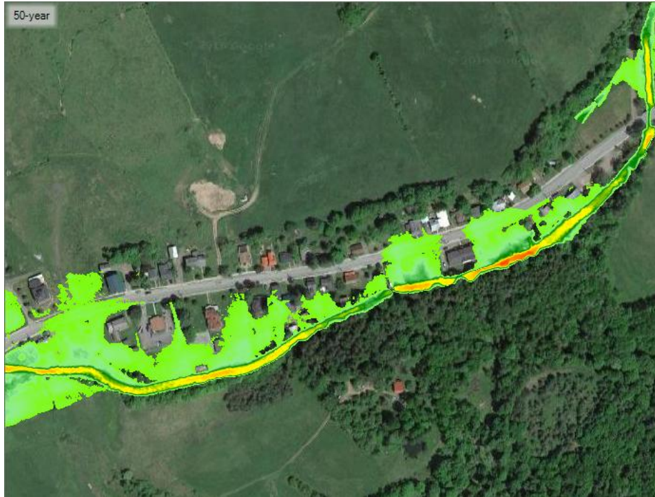
Figure 11. Inundation Area during a 50 year event for 288 Main St. to 506 Main St. – Existing Conditions
