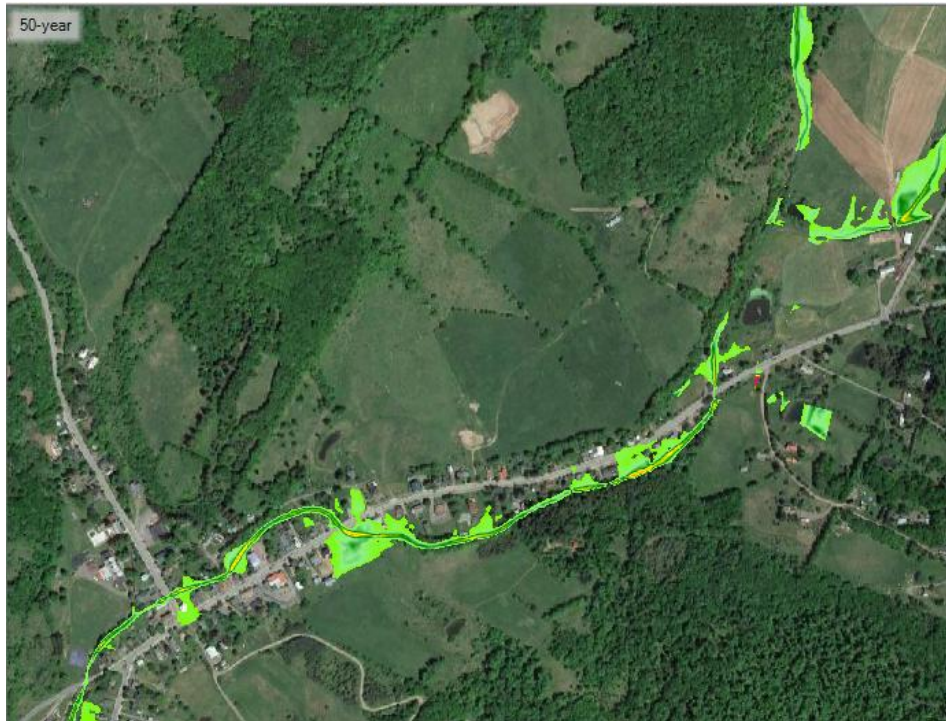
Figure 10. Inundation Area during a 50 year event - Proposed Conditions (Continuous Floodplain)
