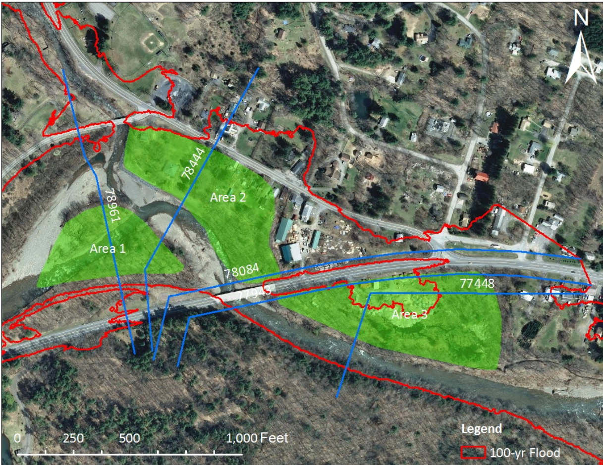
Figure 4-24 Areas of Floodplain Enhancement at the Confluence of Esopus and Bushnellville Creeks
