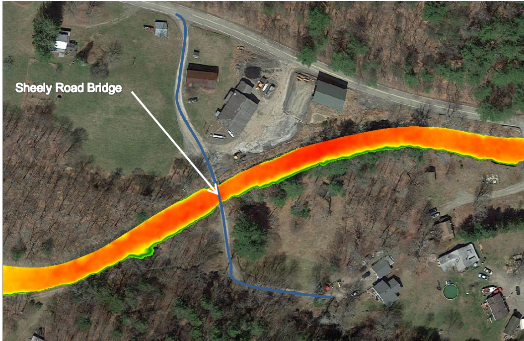
Figure 7 - Inundation Area during a 50 year event – Existing Conditions
