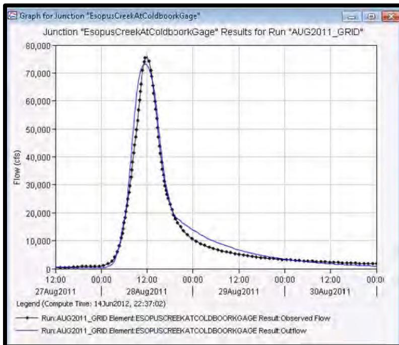
**Figure 3: Comparison of Rainfall Runoff Discharges versus Measured Discharge (FEMA 2012)**
