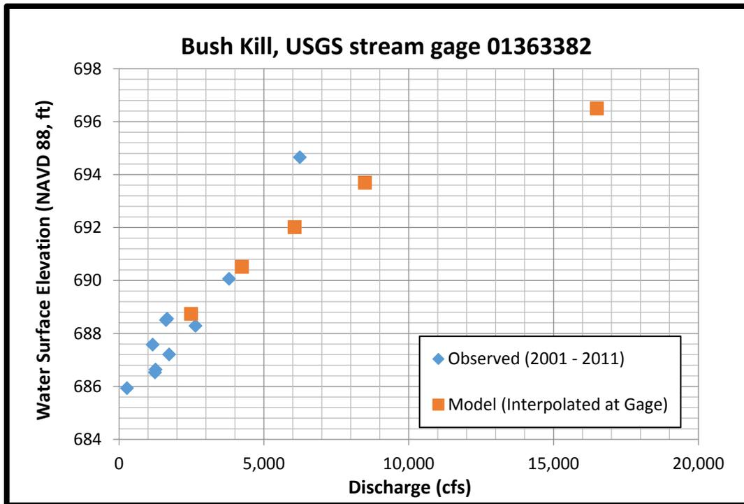
Figure 12: Comparison of Modeled Water Surface Elevations vs. Measured Water Surface Elevations.
