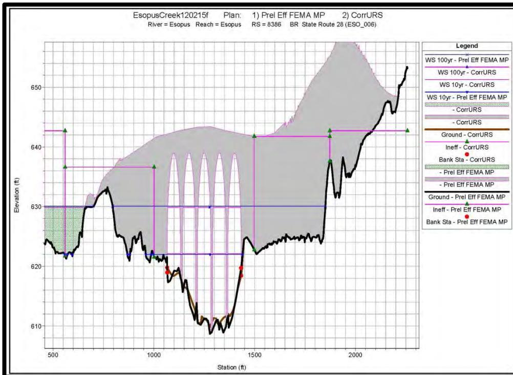
**Figure 7: Cross Section of Duplicated and Corrected Model. Note Slight Changes in Channel Topography**
