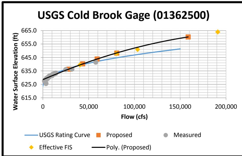
Figure 5: Comparison of Measured Discharges and Modeled Discharge in FEMA Models (FEMA 2012)
