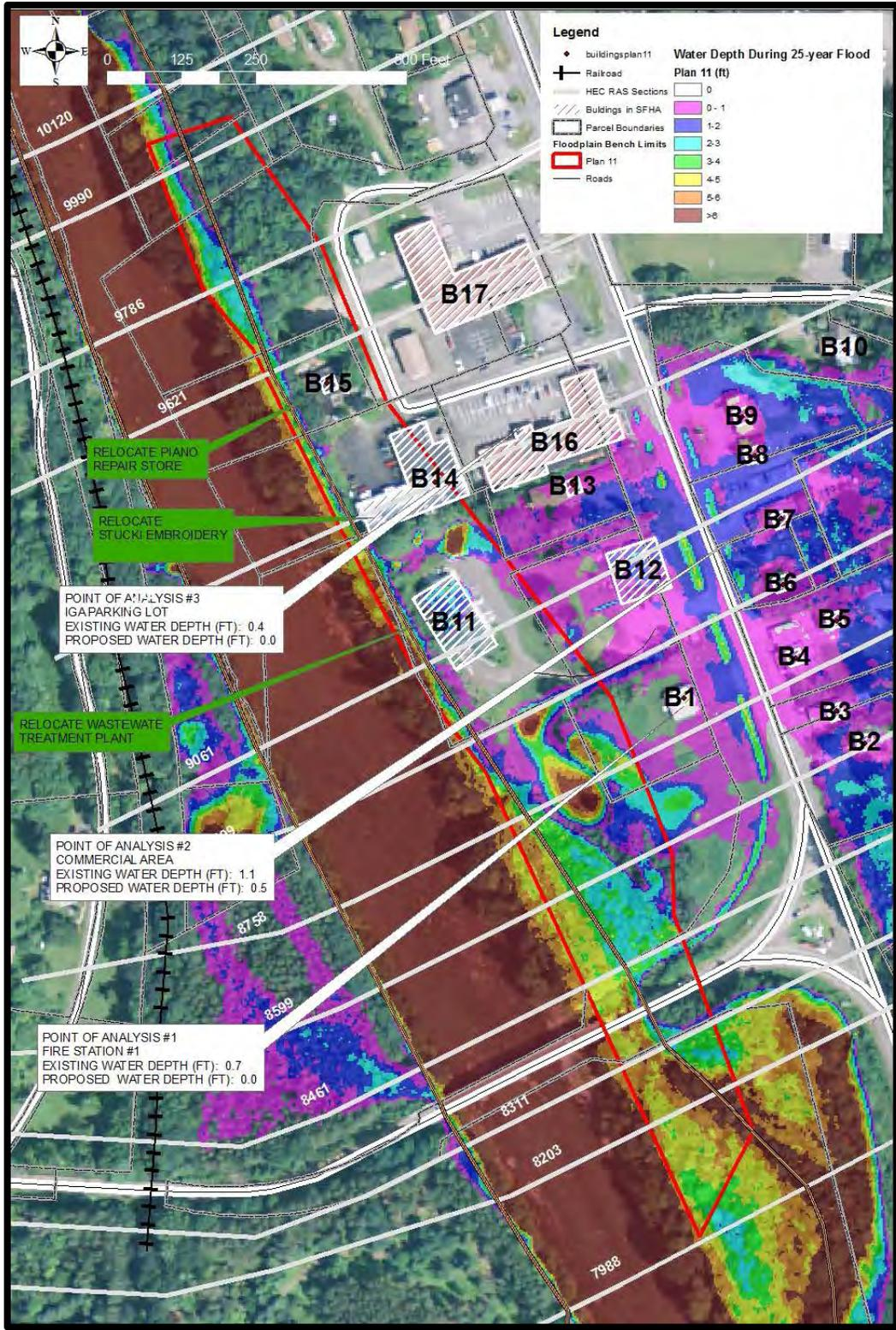
Figure 22: Conceptual Layout of Plan 11
