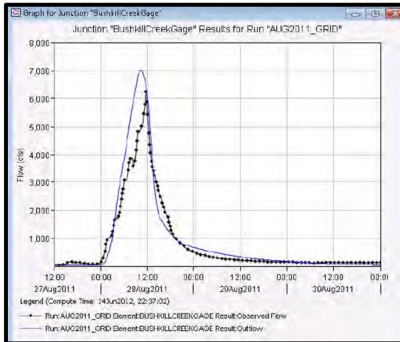
Figure 11: Comparison of Rainfall Runoff Discharges versus Measured Discharge (FEMA 2012)
