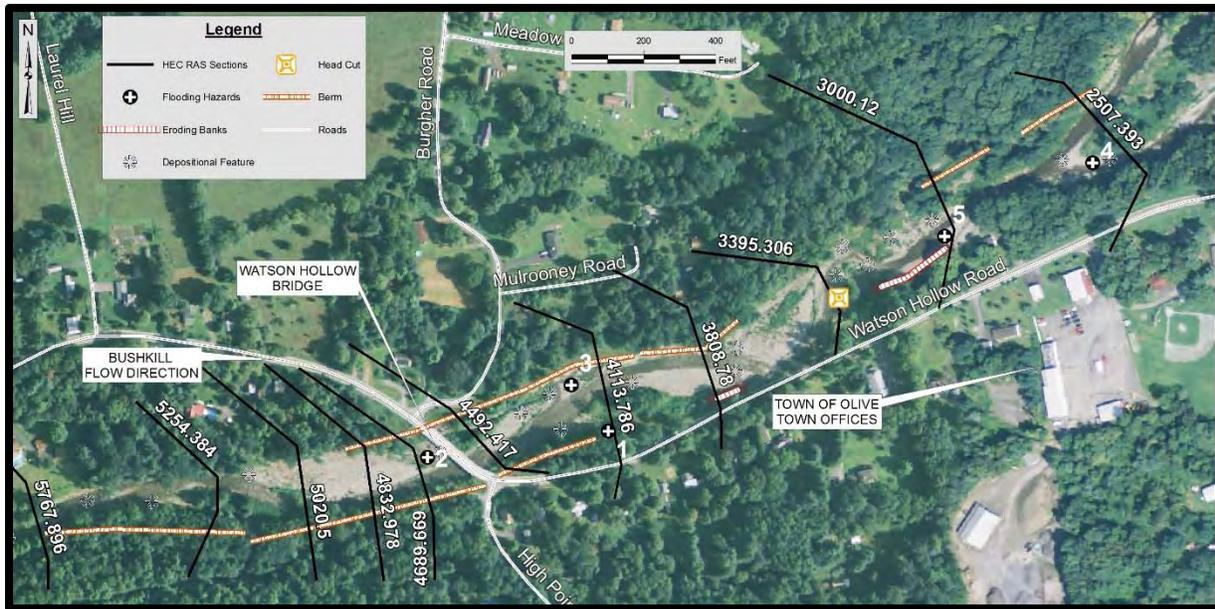
**Figure 38: Location Map of Cross Sections Used in the Hydraulic Analysis and Flood Hazards**
