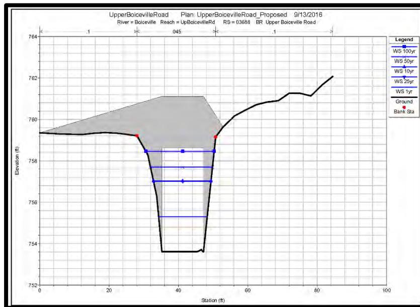
**Figure 26: Proposed Cross Section at Upper Boiceville Road Crossing**
