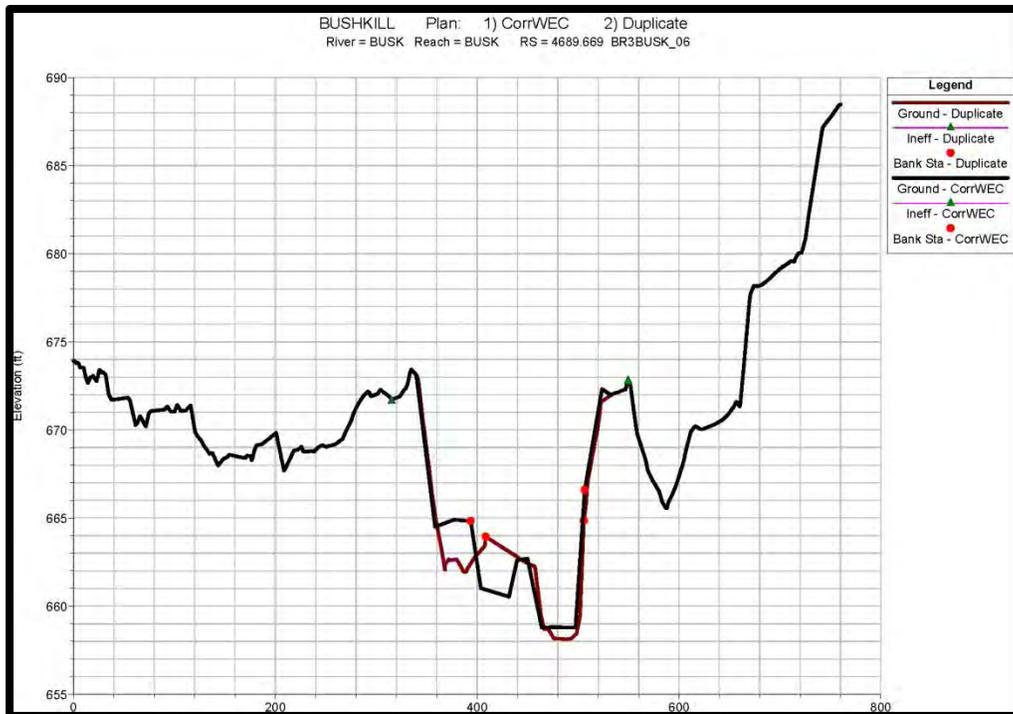
**Figure 39: Section View of the Corrected and Duplicated Topography in the Bushkill**
