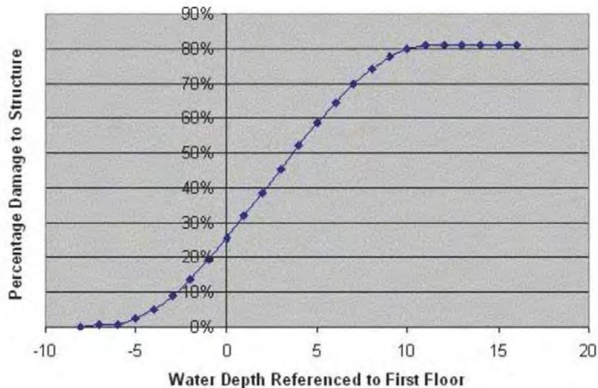
**Figure 59: Estimate of Percent Damage to a Structure Based Upon Depth of Inundation**
