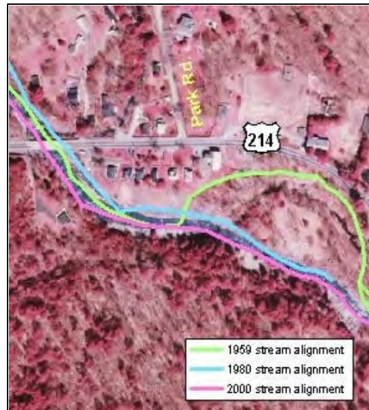
Figure 4 Historic stream channel alignments in Management Unit 18
