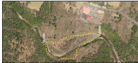
Wetland boundary approximately delineated by NWI (Stations 124840-123300)
